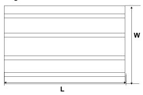
The sensors should always be mounted along the longest side of the duct, which is called the length. The shorter side of the duct is called the width.
